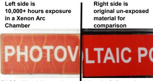
RESULTS: PASS - Material has only very slight color fading and clearly legible with no sign of adhesive failure or edge lift. Slight crackle in red ink.
