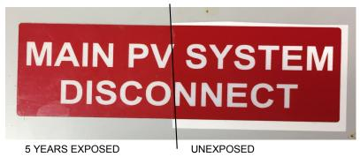
The 242 material has been tested in actual continuous outdoor exposure for five years in Wisconsin. Plate faces Southwest. After five years, the exposed label shows no signs of fading and no edge lift.
