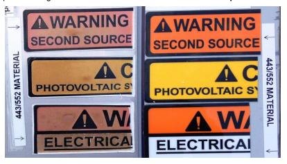
9.038 hours of exposure using Xenon Arc Slight fading of colors.
