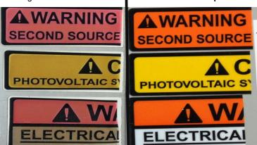
5,000 hours of exposure using Xenon Arc Slight fading of colors.
