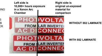
RESULTS: PASS - Material has only slight color fading and slight ink crackle on the surface. Note that the use of the 552 laminate limits UV degradation. Text is clearly legible with no sign of adhesive failure or edge lift on either sample.
