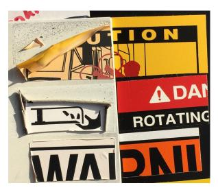
This comparison is a typical (non-HellermannTyton) silk screen on vinyl after 7782 hours of accelerated aging. (This is not a HellermannTyton product.) This test shows that thick screen print inks will fade and fail over time. 7782 hours is equivalent to 12.5 Florida Sun Years.
