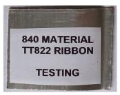
Printed samples were immersed in Gasoline for 24 hours and then a brush was applied using norml hand pressure for 10 strokes to the marked portion of the label. The label was then allowed to dry for 45 minutes and wiped 25 times with a soft cloth.
