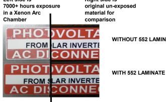
RESULTS: PASS - Material has only slight color fading and slight ink crackle on the surface. Note that the use of the 552 laminate limits UV degradation. Text is clearly legible with no sign of adhesive failure or edge lift on either sample. .
