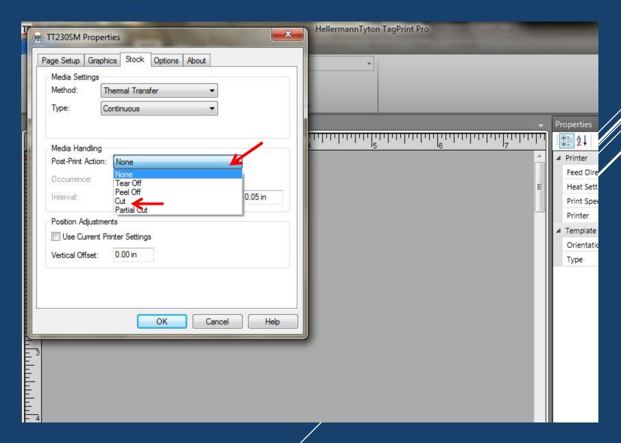
IF THERE IS NO CUTTER ON THE PRINTER, THEN LEAVE POST PRINT ACTION AS NONE. JUST CLICK "OK". IF THE PRINTER HAS A "CUTTER" CLICK ON "POST-PRINT ACTION" AND CHANGE TO "CUT" THEN CLICK OK
