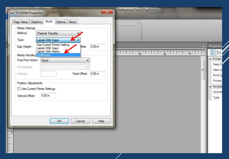
CHANGE THE "TYPE" SETTINGS FROM "LABELS WITH GAPS" TO "CONTINUOUS". IF THE PRINTER DOES NOT HAVE A CUTTER, THEN LEAVE POST-PRINT ACTION AS NONE AND CLICK OK.
