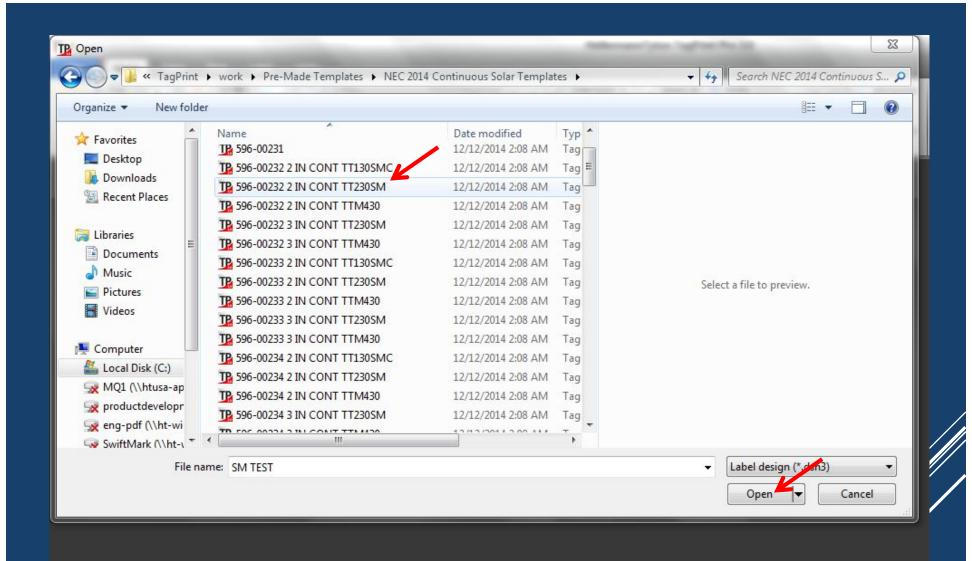
IF USING 2" WIDE PRE-PRINTED CONTINUOUS COLORED SIGNAL PANEL LABELS, SELECT 596-00232 for the TT230SM SERIES PRINTER. IF USING 3" WIDE STOCK, THEN SELECT A 3" WIDE STOCK FOR THE SAME PRINTER. CLICK TO SELECT AND CLICK ON OPEN
